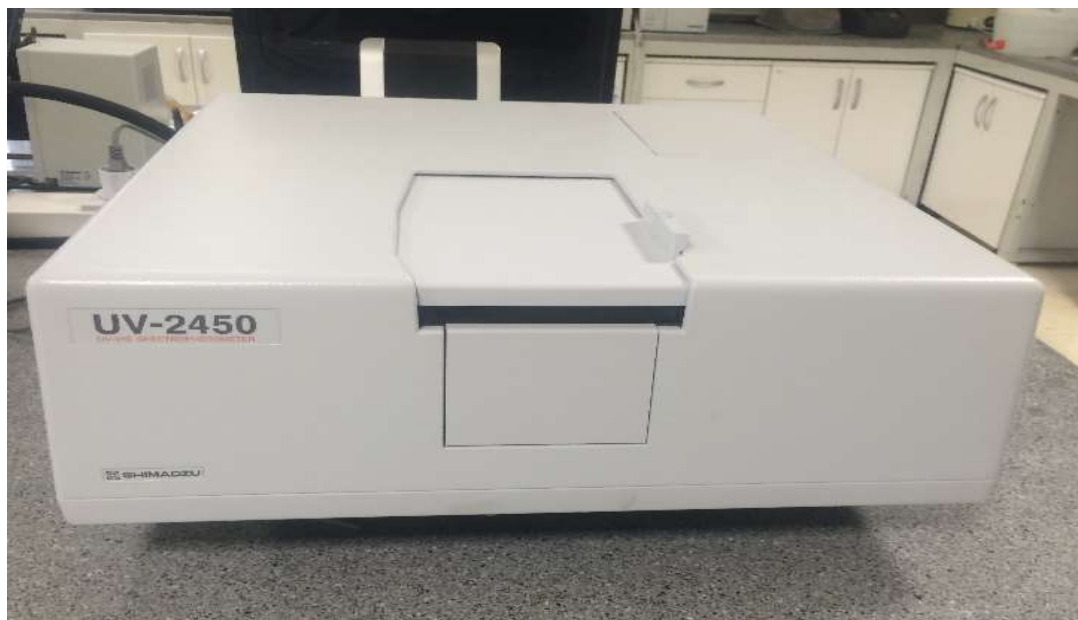
Figure 3.2 Shimadzu UV-2450 type of UV-visible spectrophotometer
