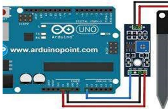
Fig 3.6: Interfacing of Moisture sensor with Arduino
