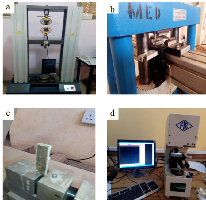
Plate 3 Testing Set-up; a) Tensile test b) Flexural test c) Impact test d) Hardness test
