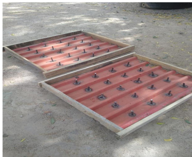
Figure 1. profiled sheets fitted with series of stud connectors.
