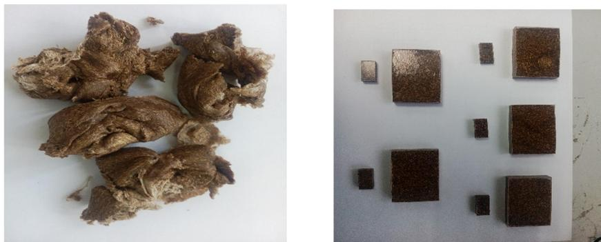
**Fig. 3: HDPE-OPEFB composite and pellets**
