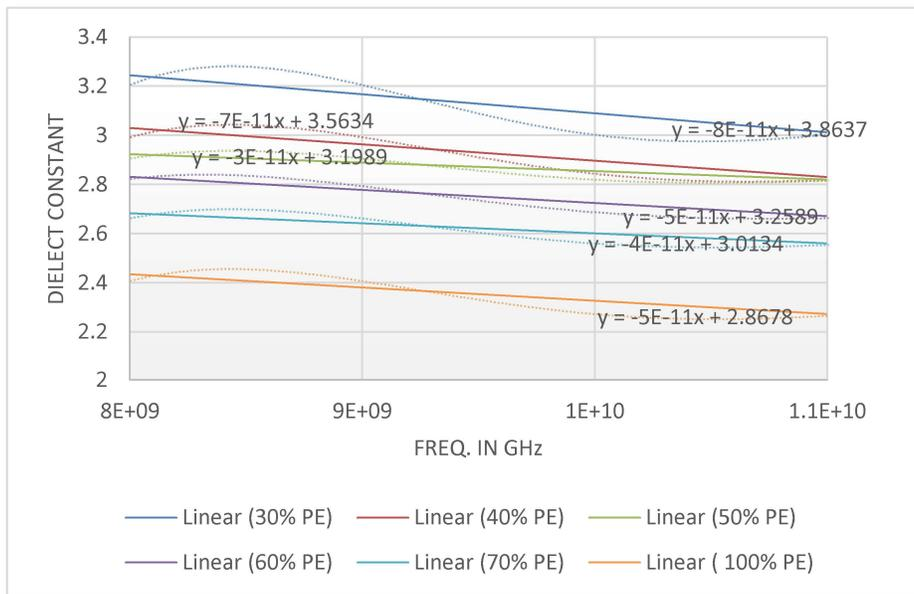
**Fig. 7: Variation of dielectric constant with frequency using RWG**
