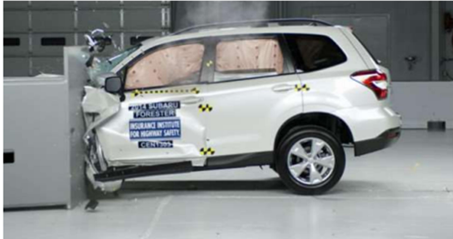
Figure 1: - frontal crash of a vehicle at a speed around 100Km/h (Patil and Patil, 2021) Car body alone was examined in this research to keep things simple. The model of the car in 3D form was generated using 3D modelling software SOLIDWORKS and the imported to the FEM analysis software ANSYS. The ANSYS workbench software was used mesh generation and also for the FEM analysis. We adopted Explicit Dynamic module and speed of the car was varied 80Km/h, 90Km/h, 100Km/h, 110Km/h and 120Km/h were selected for the crash analysis considering no difference in body dimension and material selected for the body frame.
