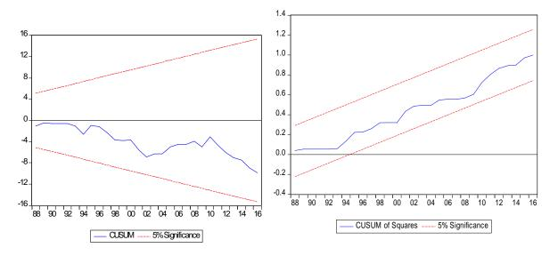
Therefore, the test is carried out using the cumulative sum and cumulative sum of squares. The result shows that our model is dynamically stable because the fitted lines fall within the dotted lines for critical value of 5%.
