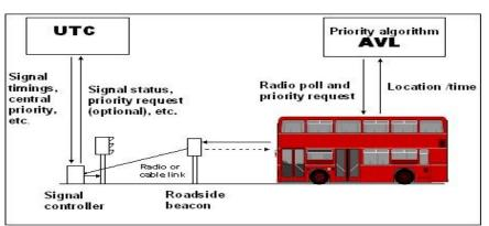
Figure 3. AVL based bus priority architecture in London
