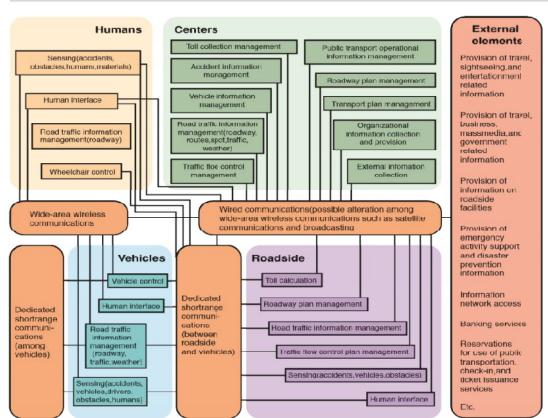
Figure 1: Subsystem Interconnect Diagram from Japanese Physical ITS Architecture Source: Yokota, T., and Weiland R.J., (2004). http://www.its-jp.org/english/arch\_e/doc/summary.pdf, p20
