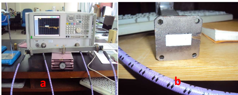
Fig. 1 (a) T/R measurement using a PNA set-up (b) Sample fitting in RWG
